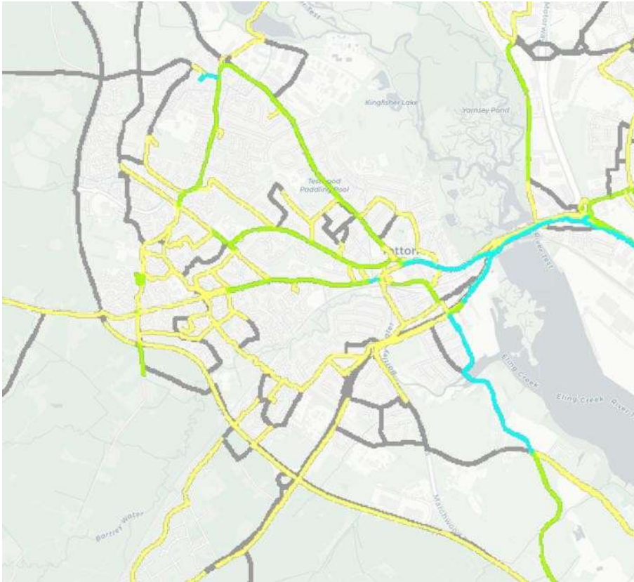
Fig. 12: pct.bike output showing routes with high (blue) and medium (green) potential demand for cycling to work – top 200 trips. Based on 2011 Census.
